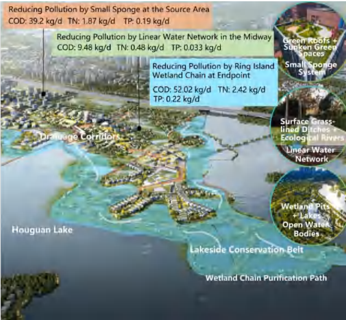
Figure 67: Schematic Diagram of the Multi-stage Ecological Pollution Interception and Purification System
