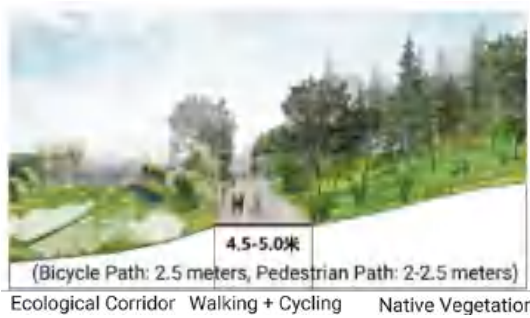
Figure 69: Cross Section of the Main Commuting Greenway
